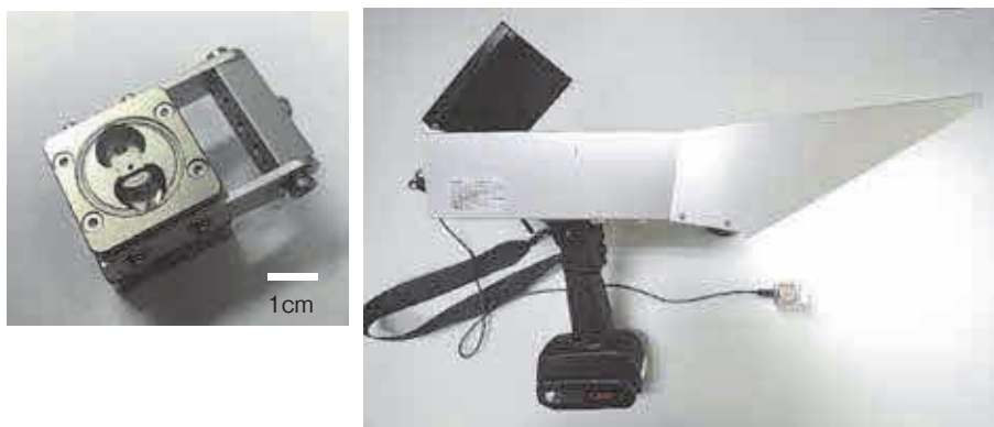
Fig. 1 Small size module used for spectroscopic analysis and installation of this module to MIJ camera available in a carcass chiller room
