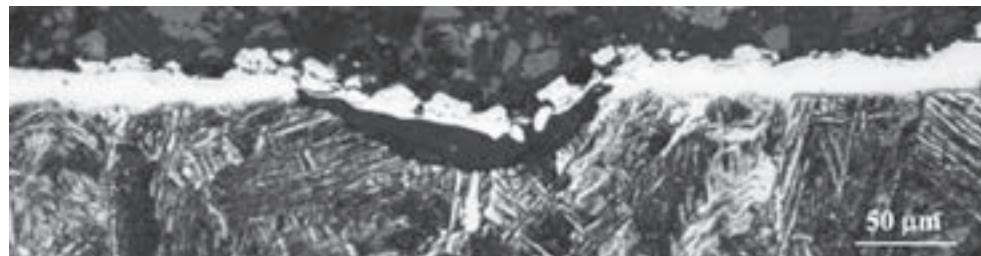
Fig. 3 Optical micrographs of corroded region
