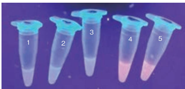
Fig. 1 The detection of Anaplasma marginal by LAMP method. No.1~3 : Positive DNA samples by PCR, No.4 : Negative DNA sample by PCR, No.5 : Negative control (Water)
