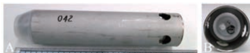
Fig. 1 Appearance of the pH sensor of a radio transmission pH measurement system. The pH sensor (A), which is 184 g in weight, 30 mm in diameter, and 145 mm in length, was composed of a small-grass electrode (B) and antenna.
