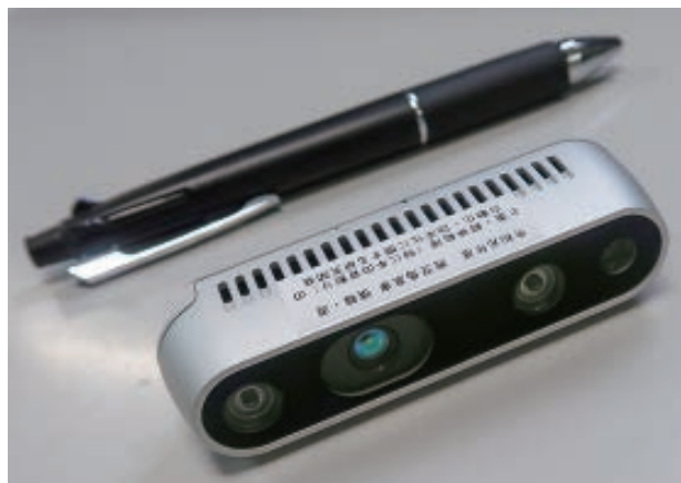
Fig.5 Intel RealSense Depth Camera D435
